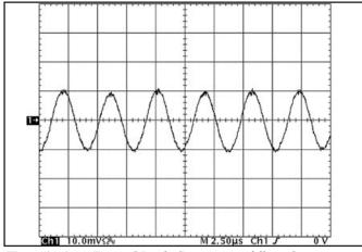
Figure 14: Input Terminal Ripple Current, i<sub>C</sub>, at full rated output current and nominal input voltage with  $10\mu H$  source impedance and  $47\mu F$ electrolytic capacitor (100 mA/div). (See Figure 13)
