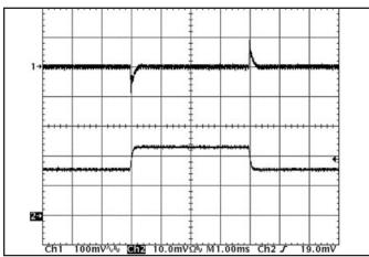
**Figure 11:** Output voltage response to step-change in load current (50%-75%-50% of lout(max);  $dI/dt = 0.1A/\mu s$ ). Load cap:  $15\mu F$ ,  $450 \text{ m}\Omega$  ESR tantalum capacitor and  $1\mu F$  ceramic capacitor. Top trace: Vout (100mV/div), Bottom trace: Iout (10A/div).
