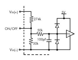
Figure B: Internal ON/OFF pin circuitry
