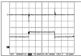
Figure 12: Output voltage response to step-change in load current (50%-75%-50% of lout(max):  $dI/dt = 5A/\mu s$ ). Load cap:  $480\mu F$ ,  $15 \text{ m}\Omega$  ESR tantalum capacitor and  $1\mu F$  ceramic capacitor. Top trace: Vout (200mV/div), Bottom trace: lout (10A/div).
