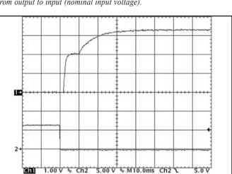
Figure 9: Turn-on transient at full load (resistive load) (10 ms/div).
